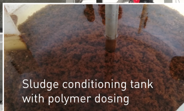
Separation of water and sludge after sludge conditioning
